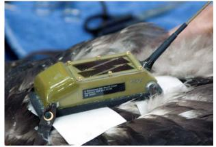
The transmitters on the eagles automatically transmit messages to Argos receivers on NOAA satellites. The satellites then transfer the messages to ground receiving stations. These stations automatically transfer the message to Argos processing centers. Then the processing centers deliver the results to the users.
